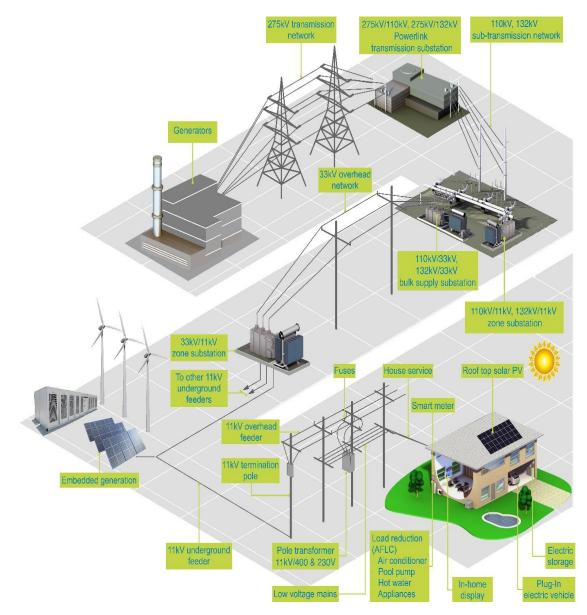
Figure 1 – Typical Electricity Supply Chain
