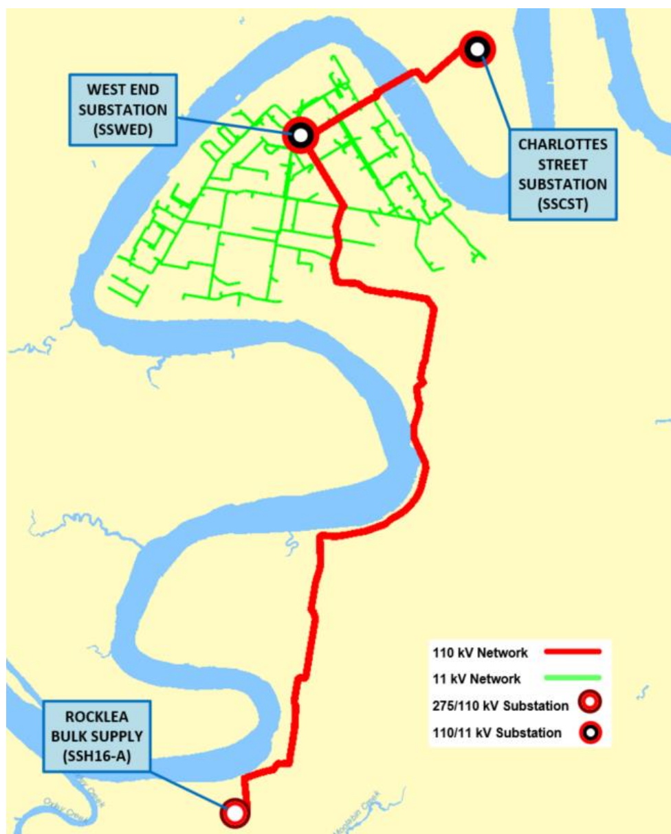
Figure 1: Existing network arrangement (geographic view).
