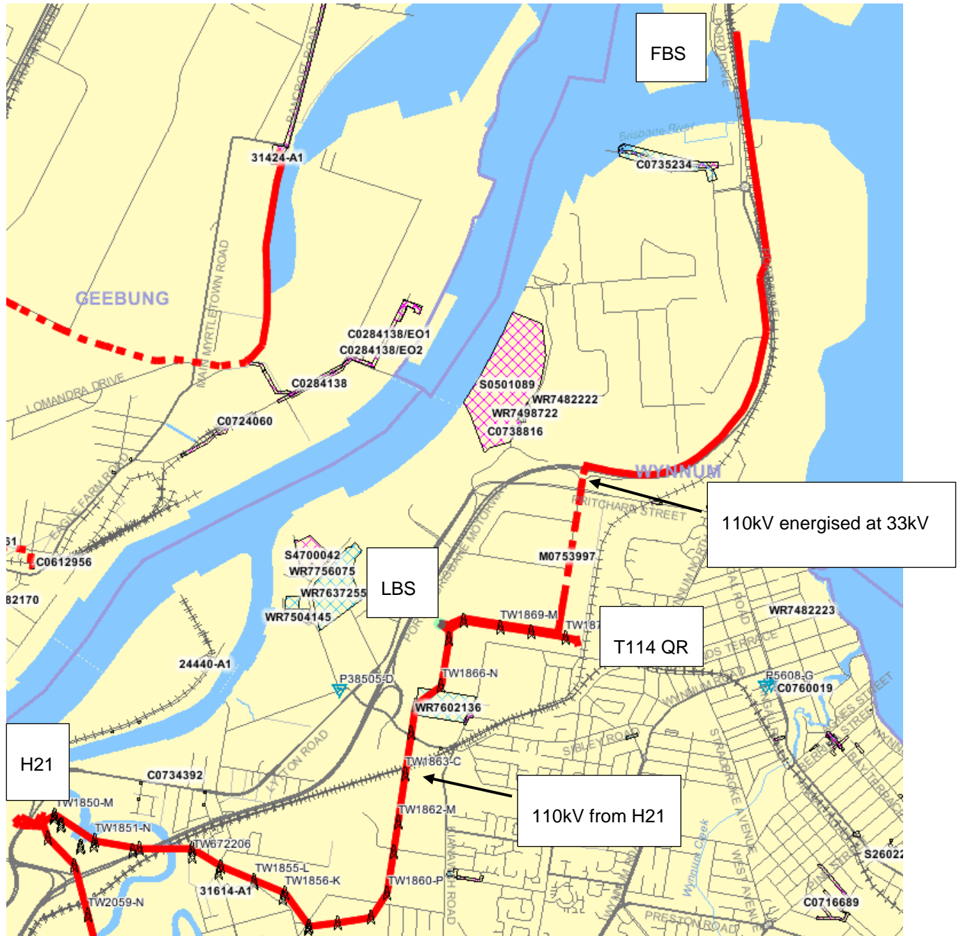
Figure 1: Existing network arrangement (geographic view)
