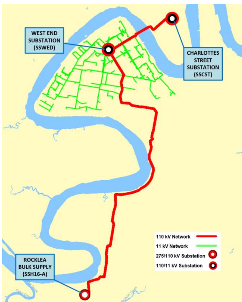
Figure 1: Existing network arrangement (geographic view).
