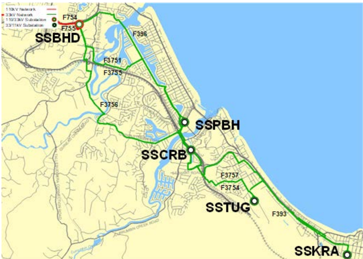
Figure 1: Existing 33kV network arrangement (geographic view)
