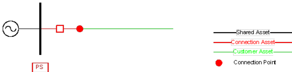
PS – Over Current feeder management for a radial load of 4MVA and above (for voltages 22/11kV).
