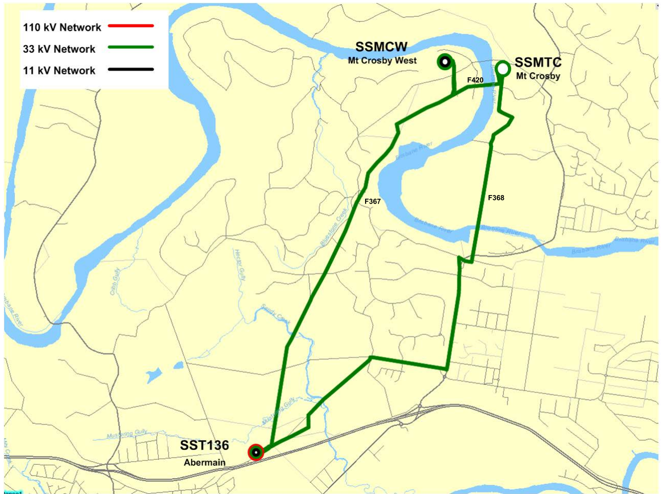
Figure 1: Existing network arrangement (geographic view)
