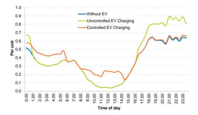
Figure 31 – Impact of Controlled and Uncontrolled EV Charging on a Residential Feeder
