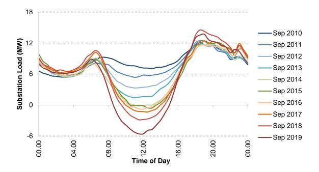
Figure 28 – Impacts of Solar PV on North Maclean Zone Substation
