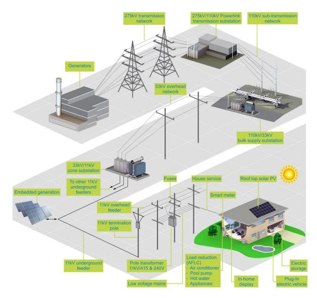
Figure 1 – Typical Electricity Supply Chain
